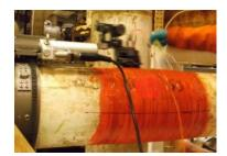
**Solution** The DRS inspection provided steel WT maps for two locations with composite repairs. The maps show two different corrosion profiles. The first location has a single isolated pit and the second shows more widespread localised corrosion. This illustrates the benefit of corrosion maps over manual spot checks which record only minimum WTs.
