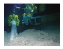
Sonomatic's ROV-deployed tools have been designed for inspecting pipelines, risers, caissons, and structural assets. The tools are adaptable, operating on both horizontal and vertical pipes Ranging from 6" to 30" diameter. A range of ultrasonic inspection techniques can be deployed, including corrosion mapping, Time of Flight Diffraction (TOFD), automated shear wave pulse echo, and component profile measurement.
