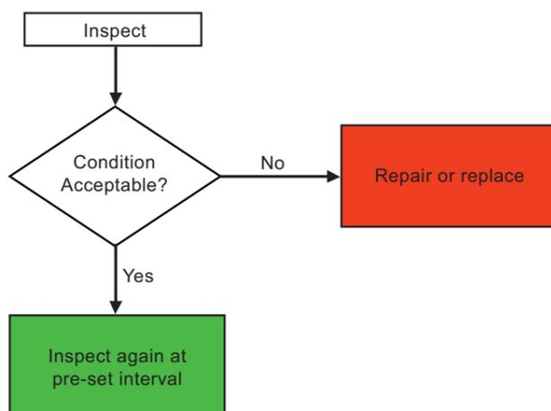
Figure 1: Historical Pipework Inspection Planning Process
