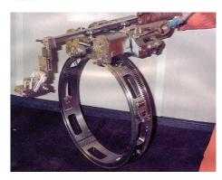
The manipulator can be applied from diameters of 150mm and above, including flat plate and cover a wide range of component geometries. The axial stroke is dependent on the application and access, but stroke lengths of 500mm are typically applied. The Nautilus has a low profile design which allows a minimum clearance of 120mm from the component surface.
