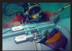
A wide variety of ultrasonic inspections techniques can be deployed, including Corrosion Mapping, Pulse-Echo angle shear wave And Time-of-Flight Diffraction. Changes from one inspection method to another can be made with the manipulator in situ, negating the time-consuming recovery of the unit to the surface.
